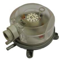
Sample Media: Field Adjustable Range: Maximum Pressure: Operating Temperature Range: Life: Automatic/Manual Reset: Connections: Casing; Air and other non-combustible, non-aggressive gases 50 Pa to 500 Pa 10 000 Pa (0.1 bar) -20 °C - 85 °C Over 10<sup>6</sup> switching operations Automatic 2 plastic pipe connection pieces, external diameter 6 mm IP54 with cover
